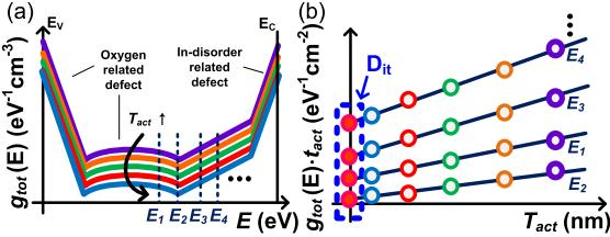
**Fig. 2.** (a) \$g\_{tot}\$ versus energy for various \$T\_{act}\$s. (b) Schematic illustrating the method to separate \$D\_{it}\$ and DOS.
