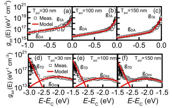
Fig. 3. Extracted  $g_{tot}$  distributions in the IGZO TFTs near  $E_C$ , with  $T_{act} =$  (a) 30 nm, (b) 100 nm, and (c) 150 nm, and near  $E_V$  with  $T_{act} =$  (d) 30 nm, (e) 100 nm, and (f) 150 nm.
