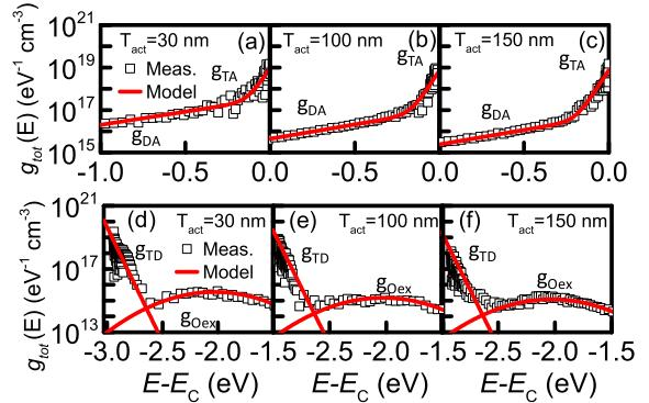
**Fig. 3.** Extracted \$g\_{tot}\$ distributions in the IGZO TFTs near \$E\_C\$, with \$T\_{act} = (a)\$ 30 nm, (b) 100 nm, and (c) 150 nm, and near \$E\_V\$ with \$T\_{act} = (d)\$ 30 nm, (e) 100 nm, and (f) 150 nm.
