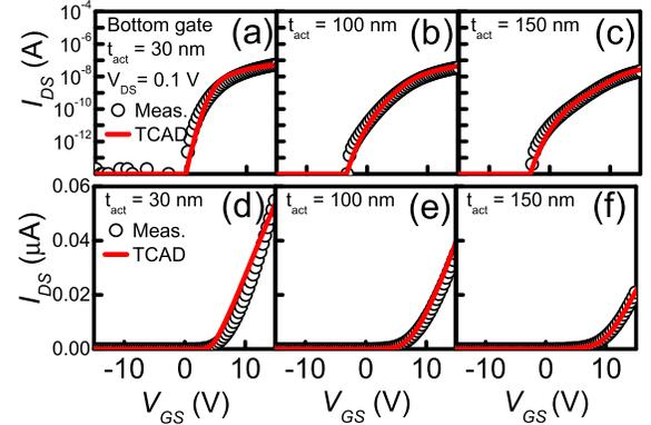
Fig. 7. Experimental and simulated  $I-V$  curves for  $V_{DS}$  under  $V_{GS} = 0.1$  V (semi-log scale: (a) 30 nm, (b) 100 nm, and (c) 150 nm; and linear scale: (d) 30 nm, (e) 100 nm, and (f) 150 nm).
