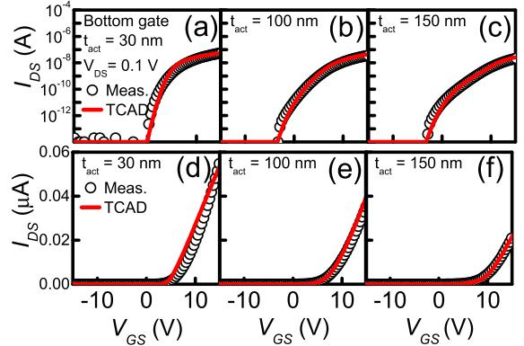
Fig. 7. Experimental and simulated  $I-V$  curves for  $V_{DS}$  under  $V_{GS} = 0.1$  V (semi-log scale: (a) 30 nm, (b) 100 nm, and (c) 150 nm; and linear scale: (d) 30 nm, (e) 100 nm, and (f) 150 nm).
