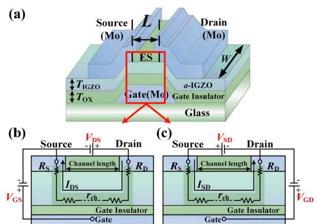
Fig. 1. (a) Schematic view of a-IGZO with an inverted staggered bottom-gate structure. Cross-sectional view and equivalent circuit for a-IGZO TFTs with  $R_S$  and  $R_D$  in (b) the forward operation mode and (c) the reverse configuration.
