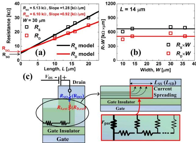
Fig. 3. (a)  $L$ -dependence of extracted  $R_S$  and  $R_D$  and (b)  $W$ -independence of normalized  $R_S$  and  $R_D$  in a-IGZO TFTs. (c) The current spreading phenomenon under the contact region.
