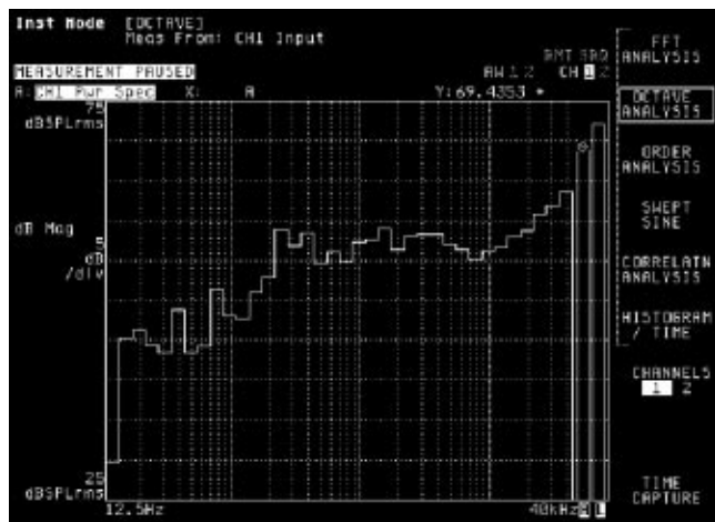
Real-time 1/3-octave measurements at frequencies up to 40 kHz.
