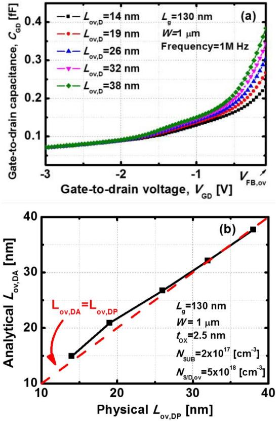
Fig. 2. (a) Simulated \$C\_{\text{GD}}\$–\$V\_{\text{GD}}\$ characteristics for various \$L\_{\text{ov},D}\$ in an n-channel MOSFET with \$W/L = 1/0.13 \text{ } [\mu\text{m}/\mu\text{m}]\$ when \$V\_{\text{GD}} < V\_{FB,\text{ov}}\$. (b) Comparison of the physical (obtained from experimental data) \$L\_{\text{ov},D}\$ and \$L\_{\text{ov},D}\$ calculated by the analytical charge model for various \$L\_{\text{ov},D}\$.
