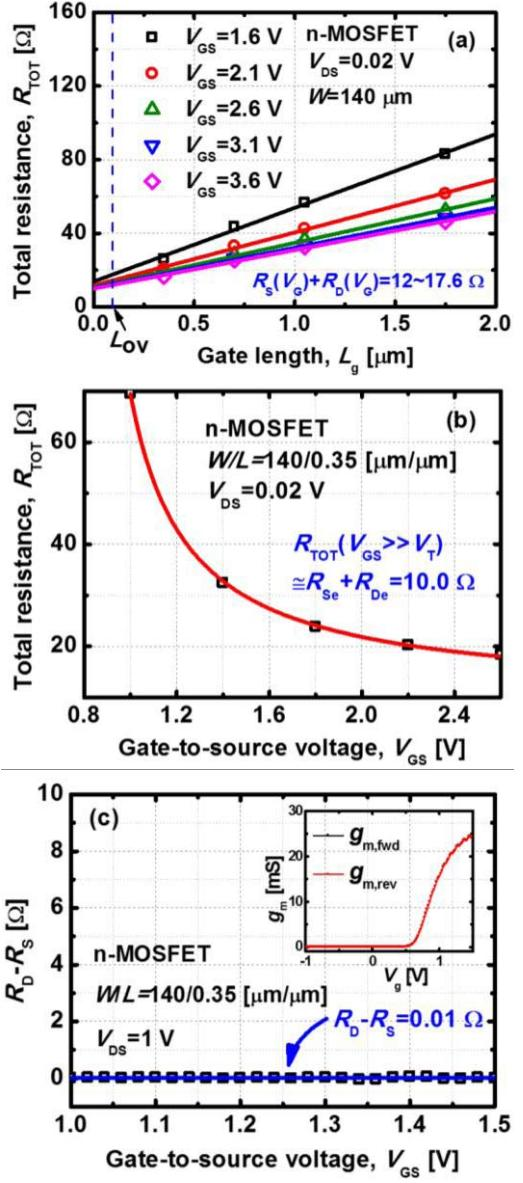
Fig. 4. (a)  $R_{TOT} - L_g$  for the extraction of  $R_S + R_D$  with  $V_{GS} = 1.6 \sim 3.6$  V. (b)  $R_{TOT} - V_G$  for the extraction of  $R_{Se} + R_{De}$  in n-MOSFET with  $W/L = 140/0.35$  [ $\mu\text{m}/\mu\text{m}$ ]. (c) Extracted  $R_D - R_S$  using the dual-sweep combinational transconductance technique. Inset shows  $g_m$  in forward and reverse modes.
