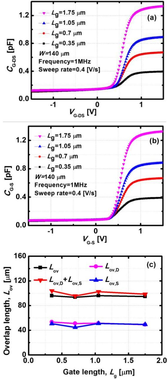
Fig. 3. Measured (a)  $C_{G-DS}$ - $V_{G-DS}$ , (b)  $C_{G-S}$ - $V_{G-S}$  characteristics of an n-MOSFET with  $W/L = 140/0.35, 0.7, 1.05, 1.75$  [ $\mu\text{m}/\mu\text{m}$ ]. (c) Extracted  $L_{ov}$ ,  $L_{ov,D}$ , and  $L_{ov,S}$  with various gate lengths.
