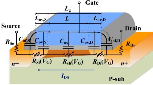
Fig. 1. Cross-sectional structure and associated equivalent circuit model with resistances and capacitances in n-channel MOSFETs.
