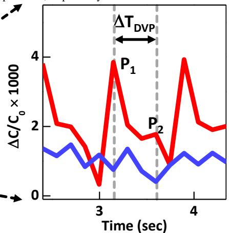
**Fig. 17** Zoom-in view of the obtained signal, which shows two peaks  $P_1$  and  $P_2$  at  $t_1$  and  $t_2$ , respectively.
