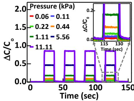
**Fig. 10** Dynamic responses of the 3D-printed pressure sensors with 80% porosity under various pressure levels.
