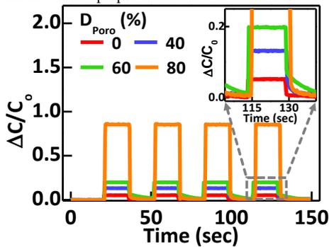
**Fig. 9** Dynamic responses of the 3D-printed pressure sensors with different porosities of 0, 40, 60, and 80% under the same pressure of 11.11 kPa.
