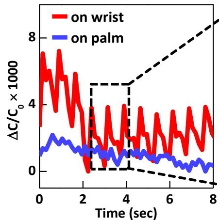
**Fig. 16** Relative change in capacitance of the 3D-printed pressure sensor with 80% porosity on the wrist and palm. The red line was measured on the wrist. The blue line was measured on the palm.
