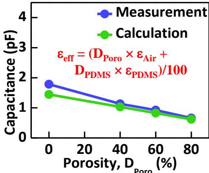
**Fig. 6** Comparison of the measured and calculated capacitance values of the 3D-printed pressure sensor with various porosities.  $D_{\text{Poro}}$  and  $D_{\text{PDMS}}$  in  $\epsilon_{\text{eff}}$  refer the volume proportions of the air and PDMS.
