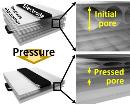
**Fig. 1** Device structure of the monolithically 3D-printed capacitive-type pressure sensor with the porous-structured dielectric before and after an external pressure was applied.
