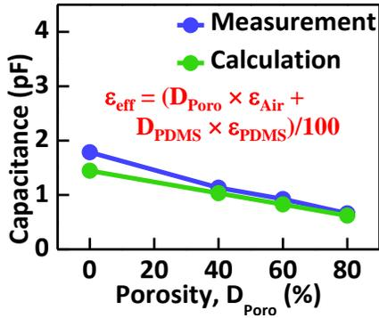
**Fig. 6** Comparison of the measured and calculated capacitance values of the 3D-printed pressure sensor with various porosities.  $D_{\text{Poro}}$  and  $D_{\text{PDMS}}$  in  $\epsilon_{\text{eff}}$  refer the volume proportions of the air and PDMS.
