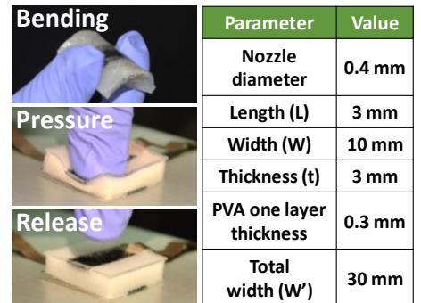
**Fig. 5** Photographs of the flexibility, softness, and resiliency of the 3D-printed pressure sensor with porous-structured PDMS. (Table I. Key parameters for the 3D-printed pressure sensor)
