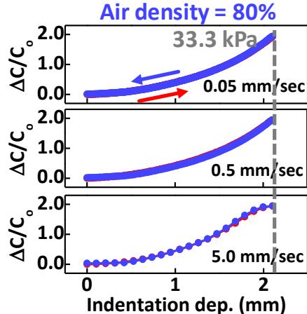
**Fig. 13** Hysteresis characteristics of the 3D-printed pressure sensor with 80% porosity in response to different sweep rates (0.05, 0.5, and 5.0 mm/sec). The red line was measured at a forward sweep. The blue line was measured at a reverse sweep.
