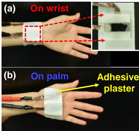
**Fig. 15** Mounting of the 3D-printed pressure sensor onto a human wrist (a) and palm (b) with commercial adhesive plaster.
