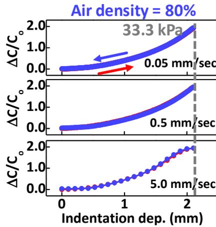
**Fig. 13** Hysteresis characteristics of the 3D-printed pressure sensor with 80% porosity in response to different sweep rates (0.05, 0.5, and 5.0 mm/sec). The red line was measured at a forward sweep. The blue line was measured at a reverse sweep.
