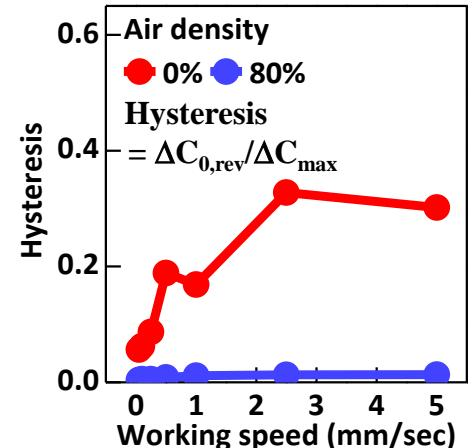
**Fig. 14** Comparison of the hysteresis performance in the sensors with the porous-structured PDMS and solid PDMS layers.  $\Delta C_{0,\text{rev}}$  and  $\Delta C_{\text{max}}$  in the equation refer to the difference in capacitance of forward and reverse sweep at 0 kPa and the maximum change of capacitance, respectively.
