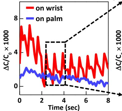
**Fig. 16** Relative change in capacitance of the 3D-printed pressure sensor with 80% porosity on the wrist and palm. The red line was measured on the wrist. The blue line was measured on the palm.
