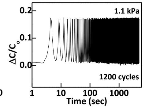
**Fig. 11** Pressure sensor reliability test (1200 cycles). In each cycle, the pressure was swept from 0 to 1.1 kPa.
