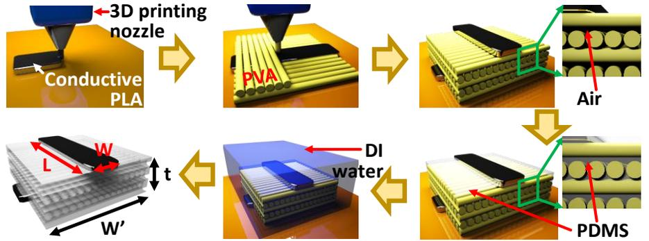
**Fig. 2** Fabrication processing steps of the monolithically 3D-printed pressure sensor with the porous PDMS layer. The flexible conductive thermoplastic (conductive polylactic acid, CPLA) was printed as the top and bottom electrodes of the pressure sensor. A polyvinyl alcohol (PVA) template was printed to form the porous PDMS layer.
