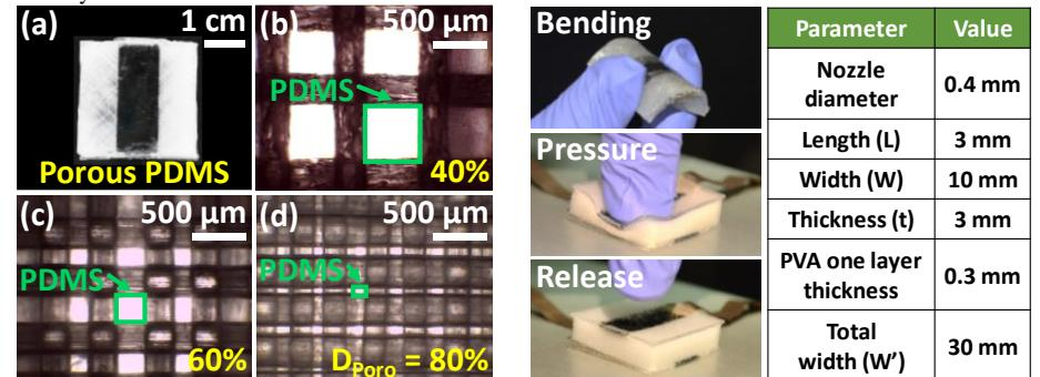
**Fig. 4** (a) 3D-printed pressure sensor after the dissolution of PVA; (b)-(d) microscope images of the porous PDMS with various porosities ( $D_{\text{Poro}}$ ) (40-80%).
