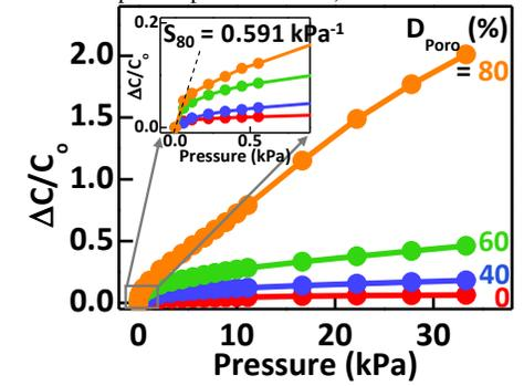
**Fig. 8** Relative change in capacitance of the 3D-printed pressure sensors with four different porosities in the PDMS (0, 40, 60, and 80%).
