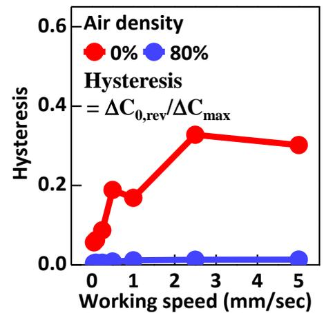
**Fig. 14** Comparison of the hysteresis performance in the sensors with the porous-structured PDMS and solid PDMS layers.  $\Delta C_{0,rev}$  and  $\Delta C_{max}$  in the equation refer to the difference in capacitance of forward and reverse sweep at 0 kPa and the maximum change of capacitance, respectively.
