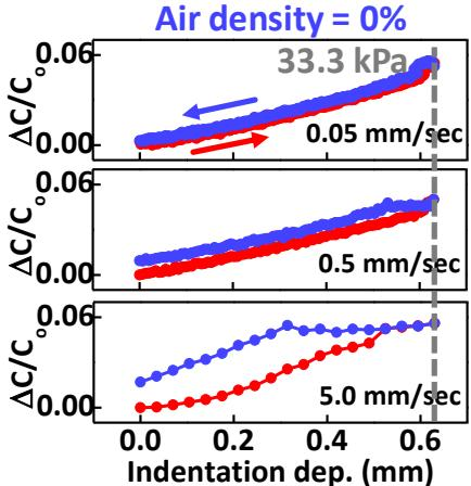
**Fig. 12** Hysteresis characteristics of the 3D-printed pressure sensor with 0% porosity in response to different sweep rates (0.05, 0.5, and 5.0 mm/sec). The red line was measured at a forward sweep. The blue line was measured at a reverse sweep.
