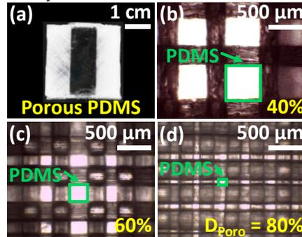
**Fig. 4** (a) 3D-printed pressure sensor after the dissolution of PVA; (b)-(d) microscope images of the porous PDMS with various porosities ( $D_{\text{Poro}}$ ) (40-80%).
