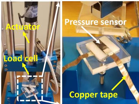
**Fig. 7** Pressure testing machine and measurement method. The copper tape was used to connect with the LCR meter to measure the capacitance changes.
