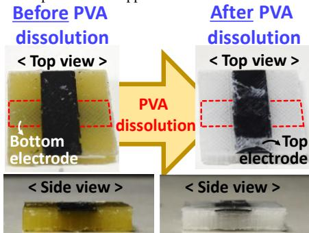
**Fig. 3** Photographs of the 3D-printed pressure sensors before and after the dissolution of the 3D-printed PVA template.
