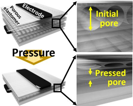
**Fig. 1** Device structure of the monolithically 3D-printed capacitive-type pressure sensor with the porous-structured dielectric before and after an external pressure was applied.
